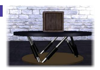
Delta has developed an RMCTools project for the RMC150 that handles communication with an external device, translates the x, y, z, roll, pitch, and yaw coordinates into cylinder positions, and controls the cylinders. This project is available from Delta Computer Systems at no charge.
