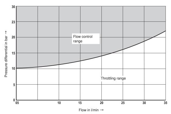
Pressure differential  $\Delta \boldsymbol{p}_{\text{min}} = \boldsymbol{p}_{\text{Pump}} - \boldsymbol{p}_{\text{Load}}$
