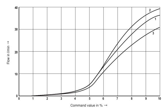
Characteristic curves measured with directional control valve type 4WRPE 6  $\dots$
