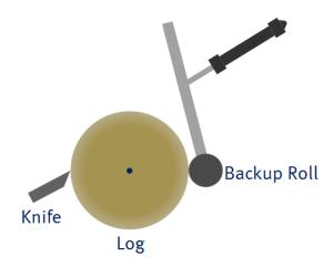
The backup roll is mounted on an arm which is moved with a hydraulic cylinder. Therefore, the
