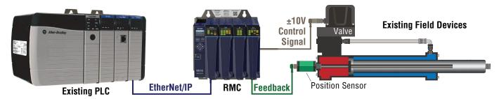
RMC Motion Controllers can duplicate the function of the discontinued ControlLogix 'analog' motion modules.
